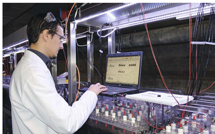
Research Assistant Maxime Blatter of the HES-SO uses electronic circuits to monitor the process and optimize electricity production and wastewater purification (Photo: Elsbeth Heinzelmann).
