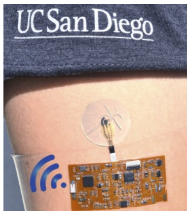
Skin-mounted microfluidic device for sweat sampling and continuous electrochemical monitoring of metabolites including a miniaturized flexible electronic board for real-time wireless data transmission (Photo by Joseph Wang, UC San Diego, USA).
